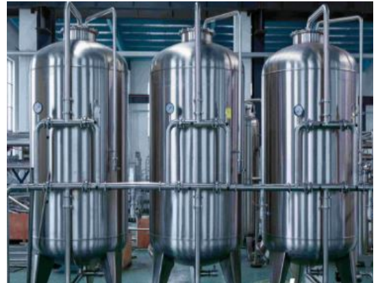
Pic.1 Water filter system
